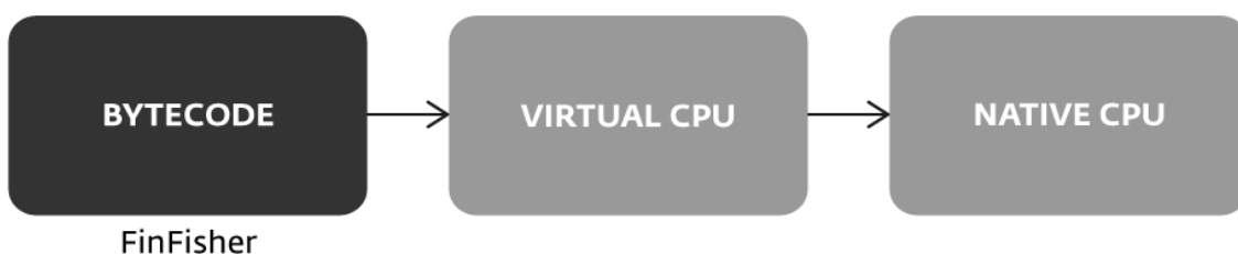
Figure 3 // Bytecode interpreted by the virtual CPU
